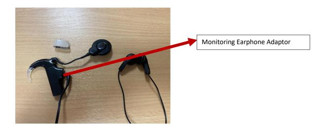
Attach the receiver between the monitoring earphone adaptor and the processor.
