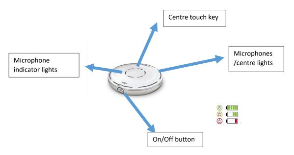
The Roger Select must be fully charged before use. Charge for three hours minimum.
